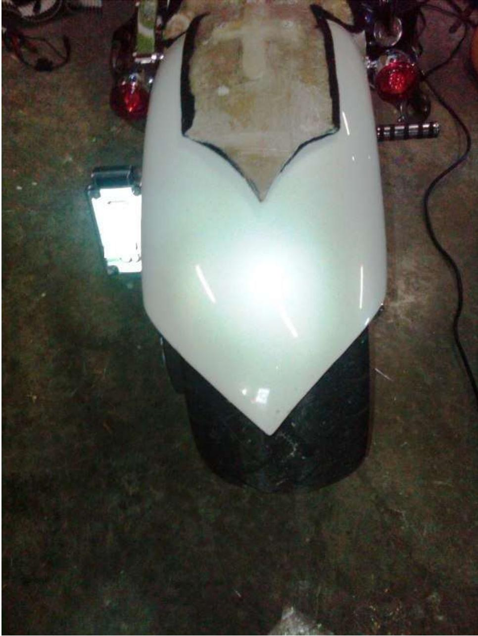
After the fact – I added a piece of sheet metal on the tail to add strength. The seat cover will be pop riveted to the pan since it is too hard to staple. I would have laid this in between the fiberglass had I thought about it prior. Oh well – live and learn...
