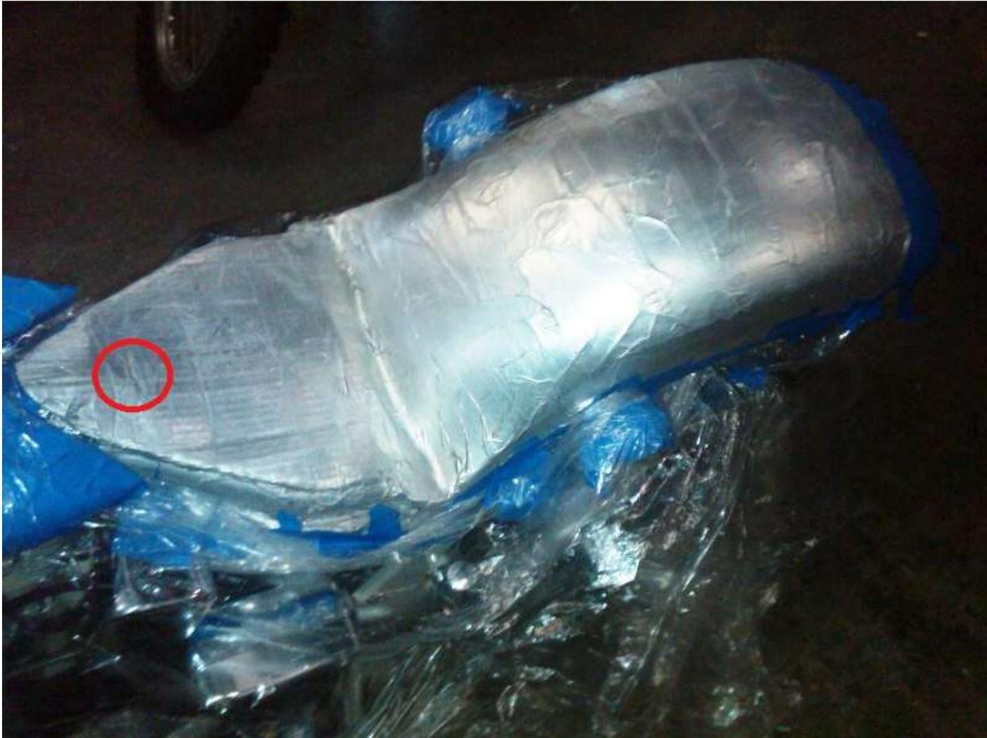
Note: You can almost see the slit I cut in the aluminum tape/cardboard for my metal tab to slide through the loop on the frame to hold the front edge of the seat. See red circle above
